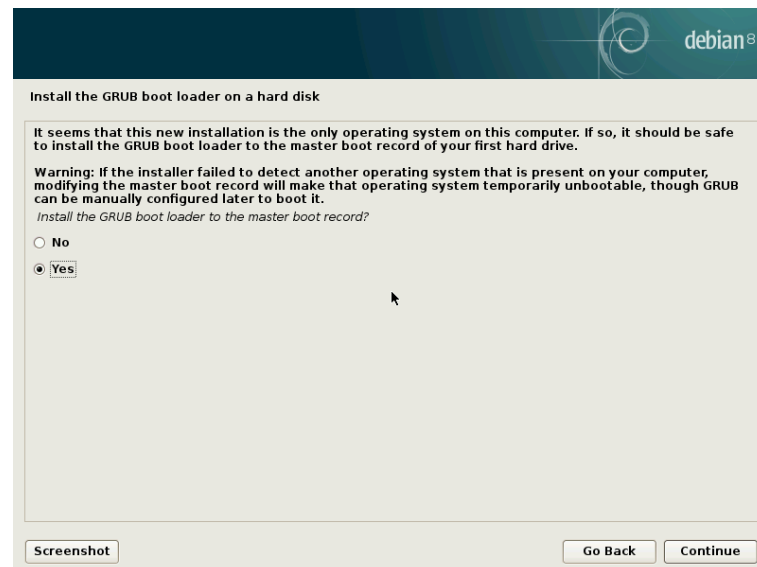
Fig. 17: Install boot loader Grub
